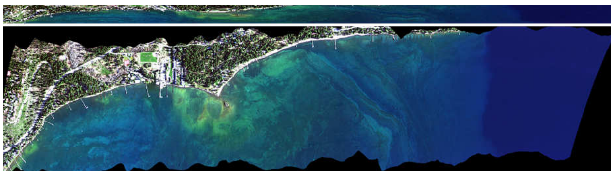
Figure 34(a). The top strip is the raw PRISM image showing along-track oversampling. This image is also available to the operator as a real time “waterfall” display. The corresponding orthorectified image is shown is of the area around the Dollar Point coast of Lake Tahoe.
