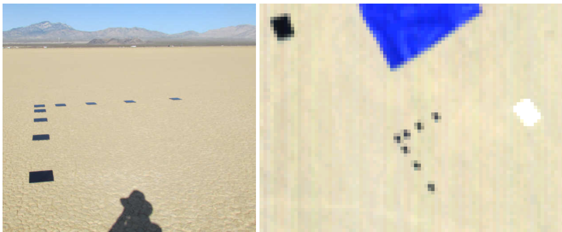
Figure 33. Left: 30 cm square spatial targets placed on the dry lakebed surface adjacent to the radiometric calibration target. Right: PRISM raw measurement showing the ability to resolve fine scale spatial targets.
