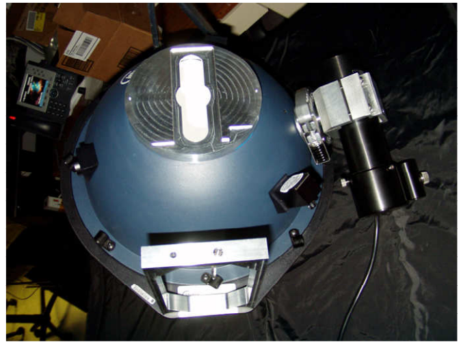
Fig. 4. Integrating sphere for radiometric and spectral calibration
