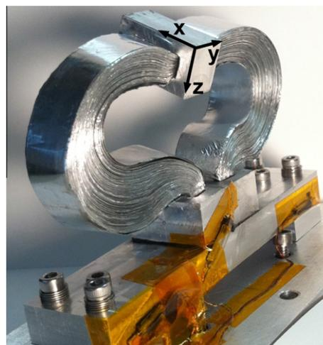
Fig. 2. TAFTS co-ordinates on the center terminal showing the base mounted silicon-diodes.
