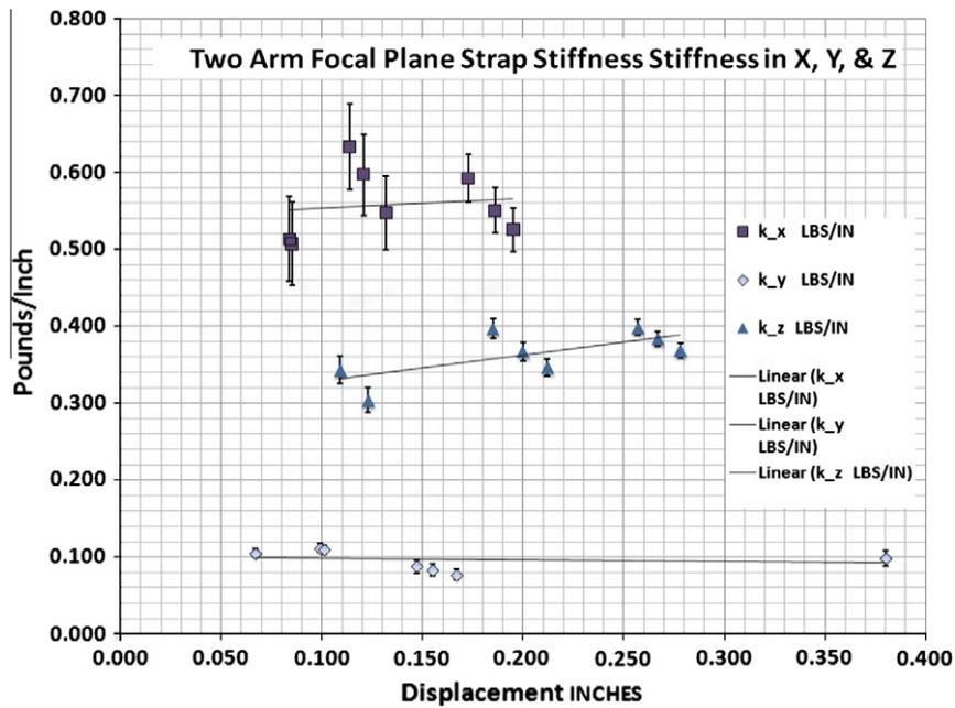
Fig. 3. Experimentally determined elasticity data for the X, Y, and Z displacements along with linear regression trendlines for TAFTS design.
