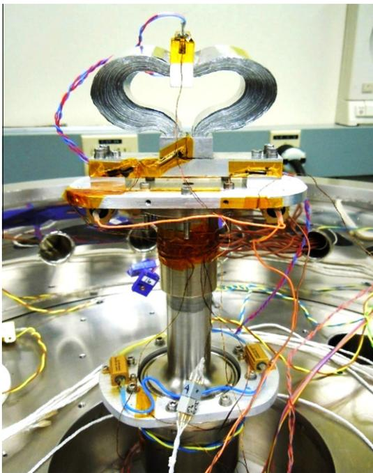
Fig. 4. The TAFTS assembly mounted on a Gifford–McMahon cryocooler at Jet Propulsion Laboratory, California Institute of Technology.
