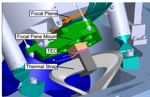
Fig. 1. TAFTS and focal-plane mount assembly on a CAD model of the PRISM instrument.
